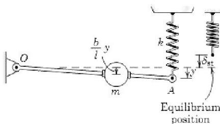
$$V = V_e + V_g = \frac{1}{2} k(y + \delta_{st})^2 - \frac{1}{2} k\delta_{st}^2 - mg\left(\frac{b}{l}y\right)$$
