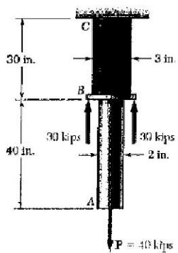
$$\text{Partion AB: } P_{AB} = 40 \times 10^3 \text{ lb}, L_{AB} = 40 \text{ in.}, d = 2 \text{ in.}$$
