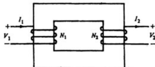
$$V_1 V_2 = N_1 N_2 = I_1 I_2 \quad .\text{۲}$$
